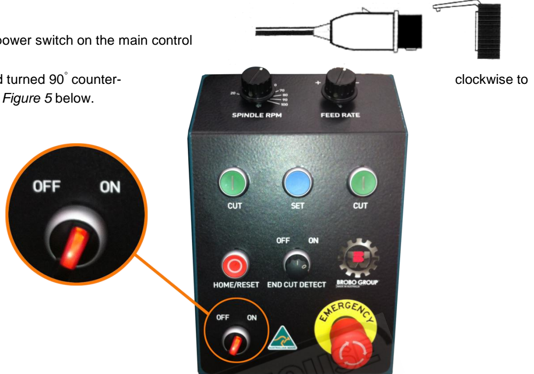
Figure 5. Power Switch on the Saw control box
